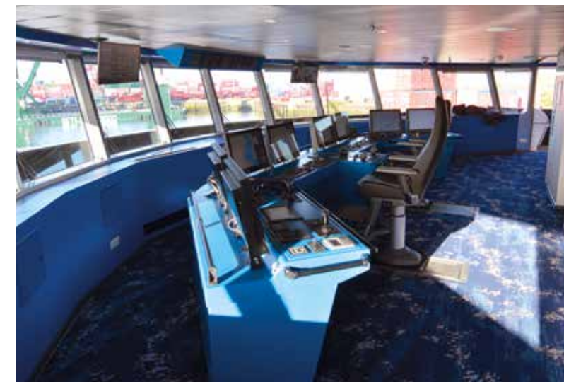
The Alpatron JRC MFD bridge contains all Navigation equipment, including the DP and thruster control systems
