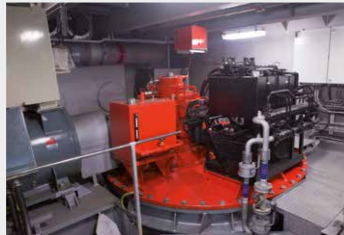
The propulsion system consists of two Veth azimuthing Z-Drive thrusters
