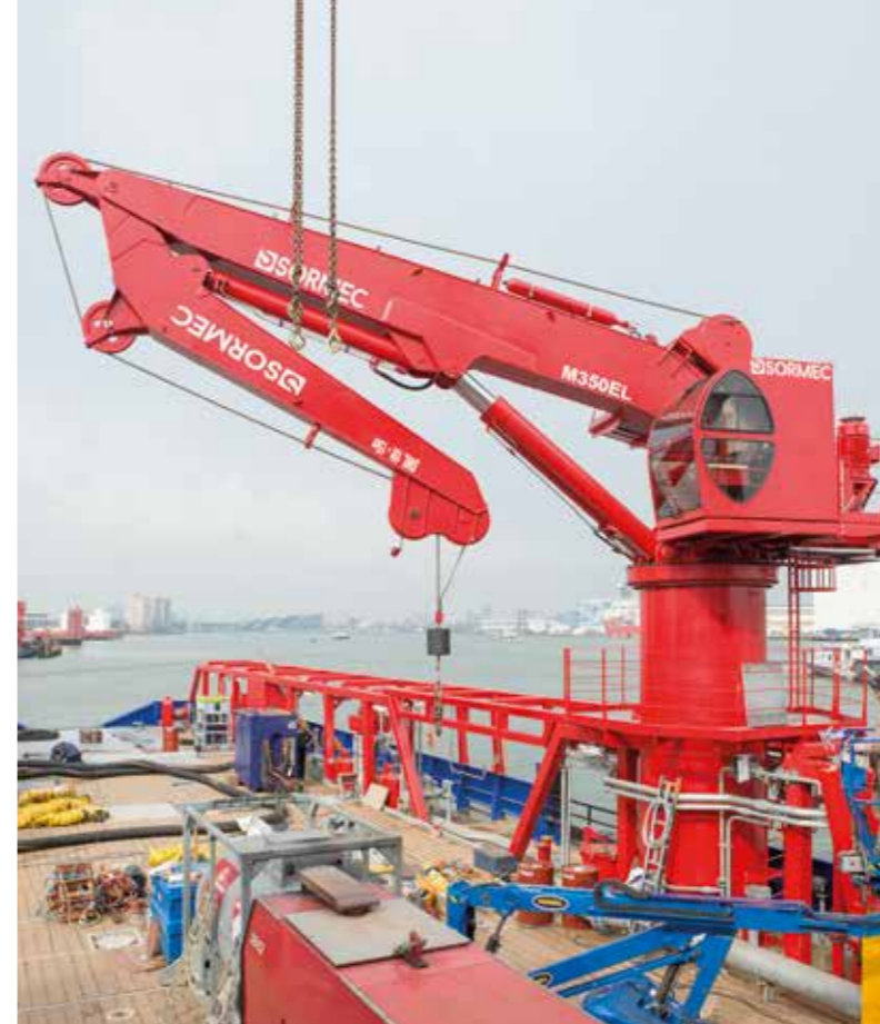
For hose handling and loading duties the OSV is equipped with two offshore knuckle boom cranes
