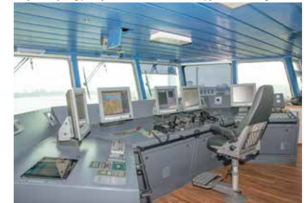
The forward facing part of the wheelhouse is used solely for transit sailing
