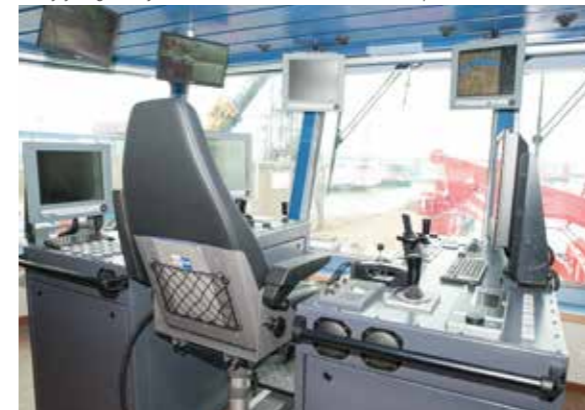
The aft facing area of the wheelhouse is where the DP assisted operations can be controlled
