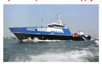
DEVELOPED FOR THE combined transport of deck cargo and passengers to offshore oil fields, the world's first hybrid propelled Fast Supply Intervention Vessel (FSIV), the Karina, exceeded expectations during sea trials this past summer.
