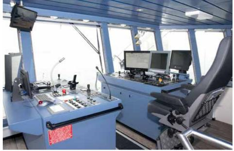
The wheelhouse aft facing area, where the DP, four-point anchoring and (un)loading can be controlled
