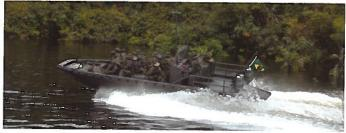
An exceptionally useful landing/assault craft, which has been built in Finland by Marine Alutech for the Austrian Ministry of Defence. This single-engined aluminium vessel is simple but immensely practical and delivers a speed of over 30 knots fully loaded.
