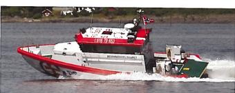
Finland's Marine Alutech, as its name implies, has until recently, specialised in aluminium vessels. This new patrol and rescue craft was its first move into FRP construction. This boat, in a tribute to the builder in particular, and Finnish boat building in general, has been delivered to the Norwegian Government rescue service.
