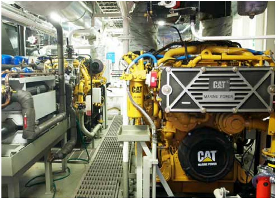
The engine room is located above the main deck, creating more space for cargo tanks below
