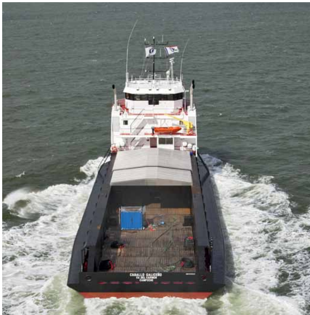
A part of the aft working deck is covered to protect the mud-processing plant from the elements
