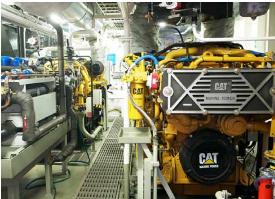
The engine room is located above the main deck, creating more space for cargo tanks below
