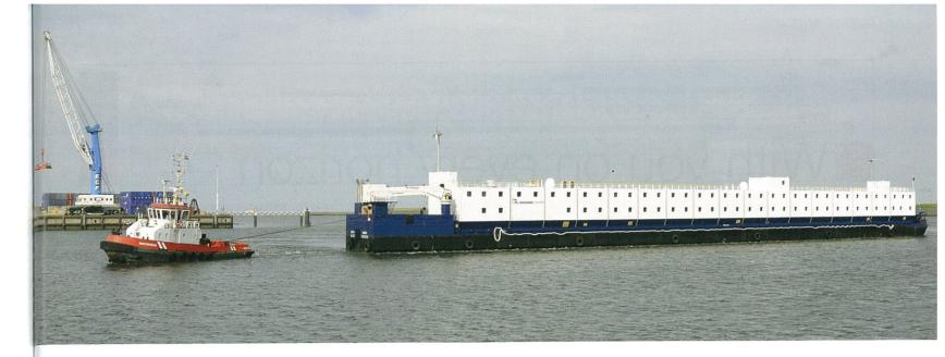
delivery the design was based on using existing newbuild inland container vessel hulls. Eventually, De Hoop built the Verdi and Holland Shipyards built the Puccini and the Bellini. The Verdi and Puccini were both delivered in December 2009, during which month Holland Shipyards also managed to deliver the Kurmangazy LQB. Built for housing 320 people, she was a conversion of the passenger vessel London Night. The Bellini was delivered in July 2010.
