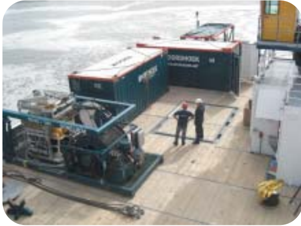
Workclass ROV spread for visual inspections
