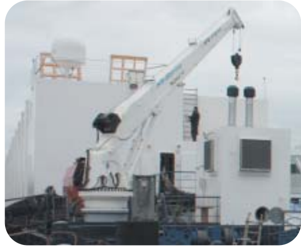
The aft deck crane can lower a 10-foot container right into the provisioning store.
