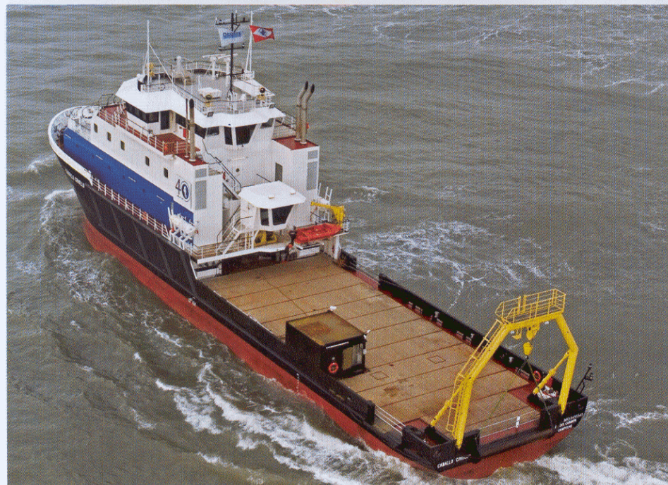
The stern-mounted A-frame is an important feature of Caballo Criollo 's outfit
