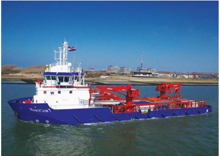
The propellers, driven by freshwater cooled electro-motors of 900kW each, are capable of producing their maximum thrust throughout a full 360-degree steering range. In the bow, two transverse tunnel thrusters, also delivered by Veth and driven by aircooled e-motors of 450kW each, are fitted. These thrusters, fixed pitch propellers operating at variable speed and controlled by a variable frequency converter, are predominantly used in DP mode and when mooring.
