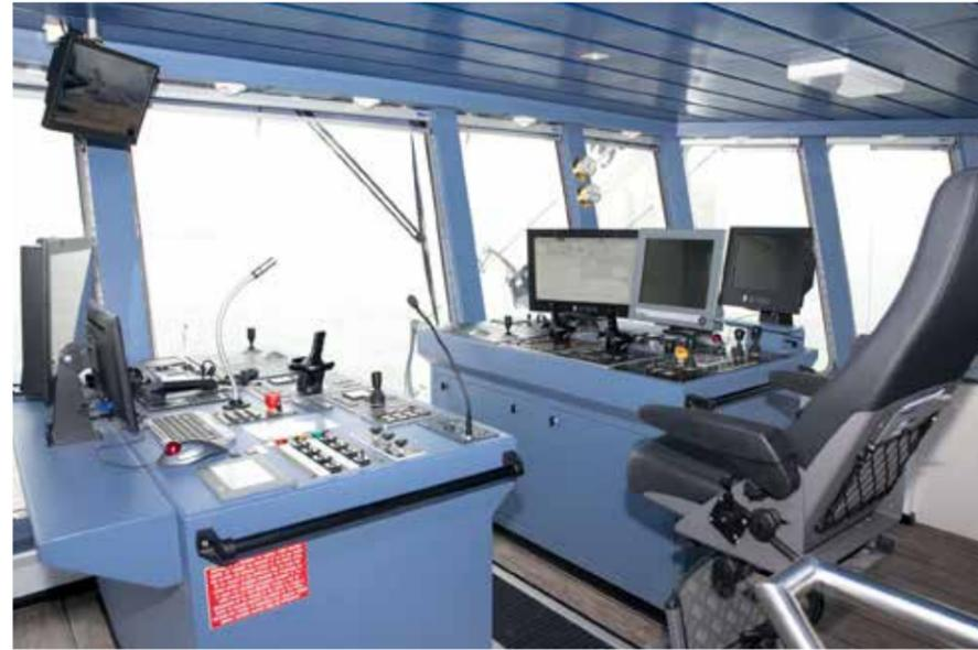
The wheelhouse aft facing area, where the DP, four-point anchoring and (un)loading can be controlled
